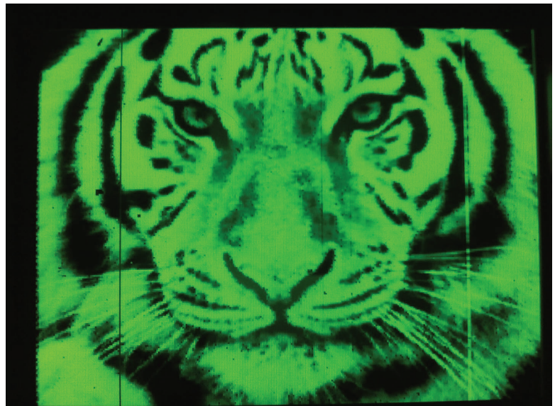
Figure 3. The QVGA AMOLET display in operation.
